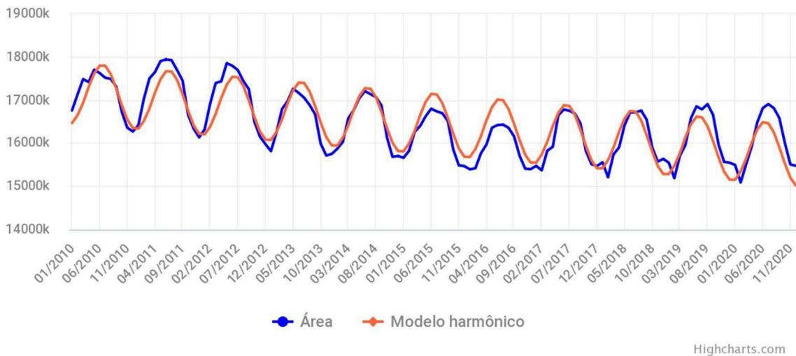
**Figure 10.** Example of fitting a harmonic series to the results of mapped monthly water surface data. The blue line is the mapped water surface area, the red line indicates the harmonic fitted model.
