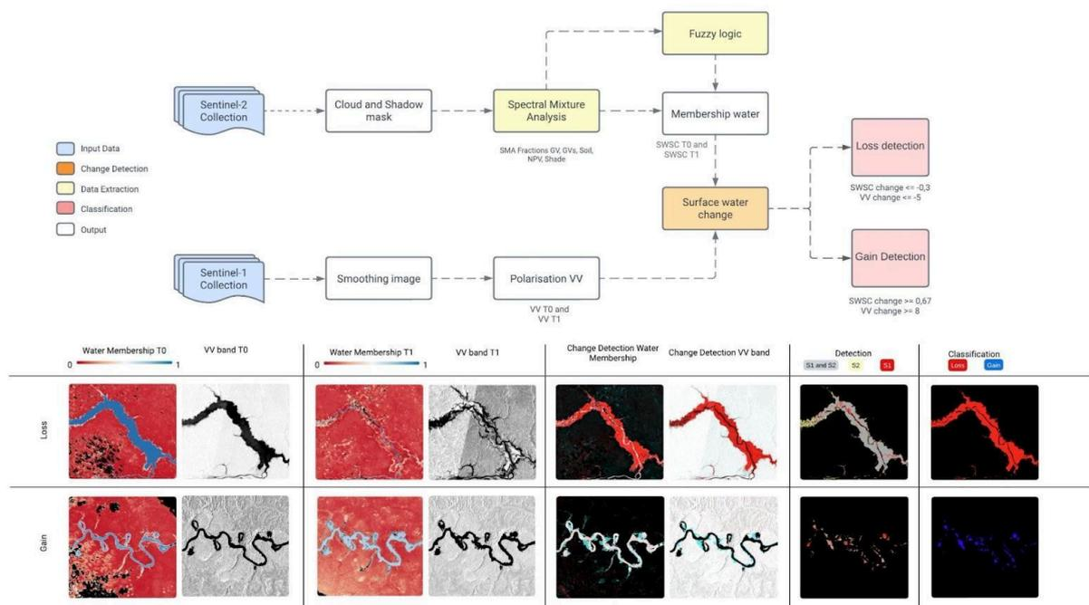
**Figure 4.** Remote sensing workflow to detect surface water change between 2022 and 2023 (i.e., loss and gain) using Sentinel-1 and Sentinel-2 satellite imagery and examples of surface water change detected with both sensors
