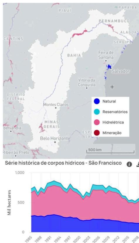
**Figure 13.** Example of water bodies classification for the São Francisco hydrographic region. The map shows hydroelectrics interrupting the natural water flux of the river in three different sectors. The graph show the area mapped as surface water among the different classes of water bodies.
