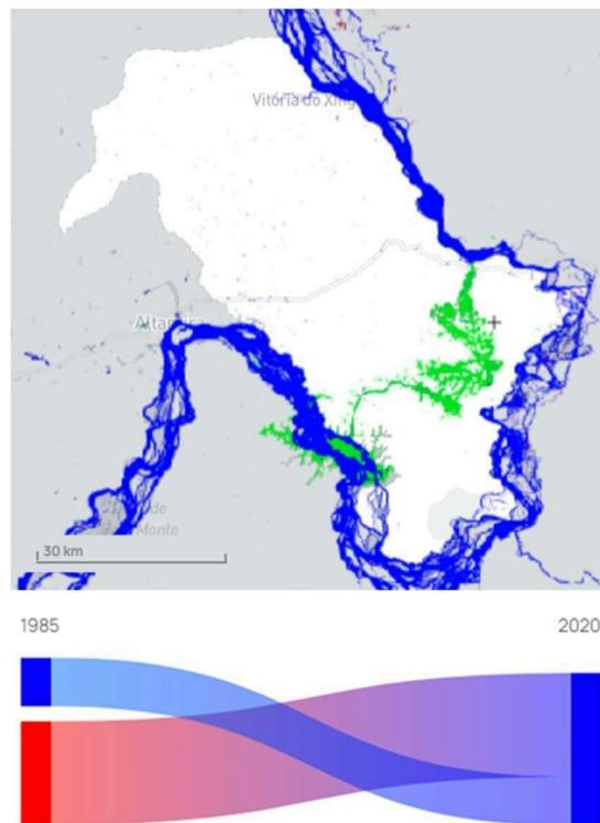
**Figure 9.** Example of surface water transitions for the Vitória do Xingu municipality. The green in the map indicates the water surfaced the appeared in the last years with the construction of the Belo Monte dam. A graph (red and blue) indicates the transition between the selected years, according to the mapped water surface area.
