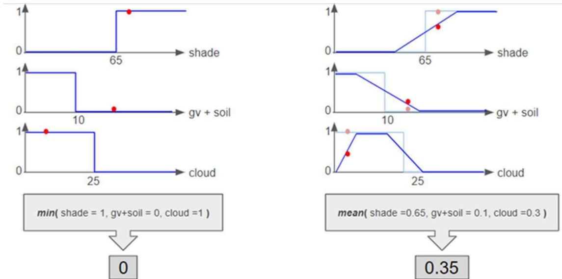
**Figure 2.** Surface Water Sub-pixel Classifier binary rules. The left example show an example of undetected surface water for a pixel with fraction values indicated by the red points (the value of  $gv + soil$  is above the threshold  $> 10$  to be classified as water). The right example applies a linear probability function to variable and the mean value allows to correctly classify the pixel (red point) as surface water.
