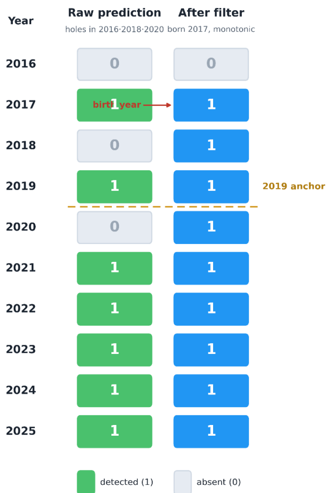
Figure 3. Temporal-consistency filter applied to a single pixel. The raw prediction (top) has spurious holes in 2016, 2018 and 2020; after filtering (bottom) the pixel is born in 2017 and remains positive thereafter. The dashed line marks the 2019 anchor.
