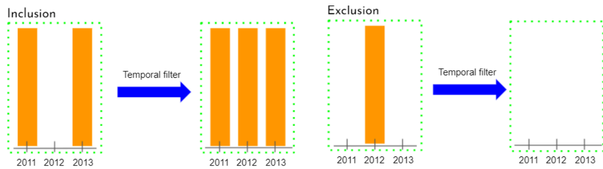
Figure 16. 3-year temporal window filter: The orange bars represent pixels of the mapped class (interest class). The exclusion filter changes a pixel to the “others” class when the same pixel was not of interest class in the adjacent years. The inclusion filter changes a pixel to the interest class when the same pixel was of the interest class in the adjacent years.
